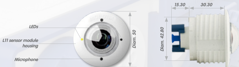
Dimensions of S14D L11 Sensor Module
