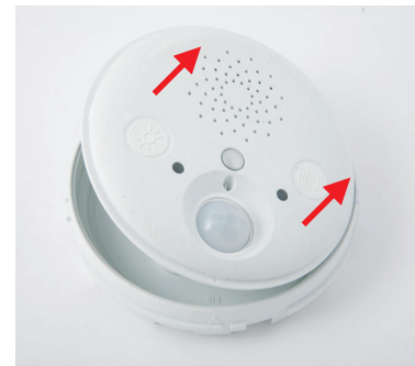
Remove the back of the housing
