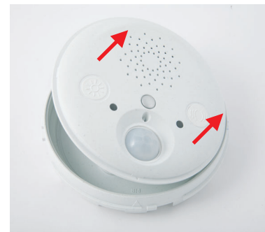
Remove the back of the housing
