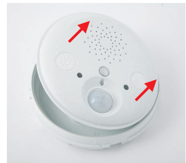
Remove the back of the housing
